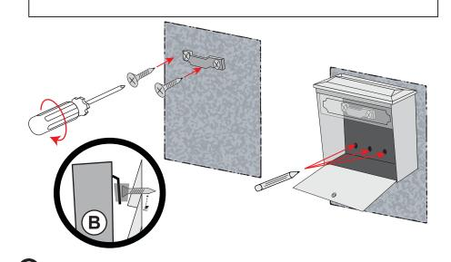
Using a masonry style drill bit(not provided), drill the bottom three pilot holes approximately 2 inches deep into the wall material. Now hang the Townhouse from the mounting bracket and secure to bottom using three 21/4" screws provided. Be sure to put some weather resistant caulk into the holes. If your wall is a thick brick, stucco or concrete you will may need masonry screws or anchors for attachment, consult a contractor if necessary.
