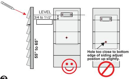
Using a 1/8" drill bit, drill the top two pilot holes approximately 2 inches deep into the the wall material. Attach the mounting bracket using the two 21/4" screws provided. Be sure to put some water resistant caulk into the holes. Now hang the Townhouse from the bracket as shown in figure **A** next mark the bottom three holes with a pencil.
