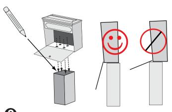
Using a 1/4" drill bit, drill four pilot holes in the marked positions approximately 1 1/2" deep into the wood. Attach the Townhouse to the post using four 1 ½" lag screws. A ½"drive socket or a ½" wrench may be used.
