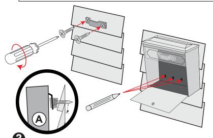
Using a 1/8" drill bit, drill the bottom three pilot holes approximately 2 inches deep into the wall material. Now hang the Townhouse from the mounting bracket. If there is a large gap between the Townhouse and the wall, insert a bushing on the screw between the back of the box and the mounting surface as shown in figure **C**. Insert some water resistant caulk into the hole and secure to bottom using the remaining three 21/4" screws provided.
